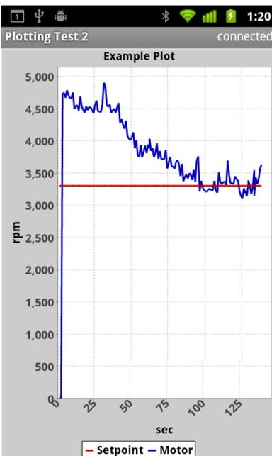
The final example using this raw data, will plot all the fields. Setpoint rpm with Motor rpm on one chart and the Drive pwm on another.
